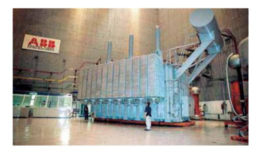
Before finalising their choice of transformer, Escelsa's Project Management unit evaluated 16 different configurations, including both single-phase and treephase transformer banks and various insulation options. Total configuration owning cost, reliability of the equipment, solutions to the problem of different secondary voltages in the regions to be connected and shortest possible reconnection time, were the main factors taken into consideration.
